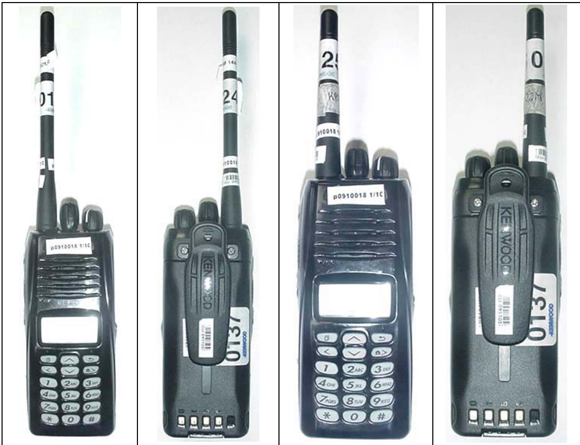
Front & Back of DUT with KRA-26M Whip Antenna Front & Back of DUT with KRA-22M Stubby Antenna
