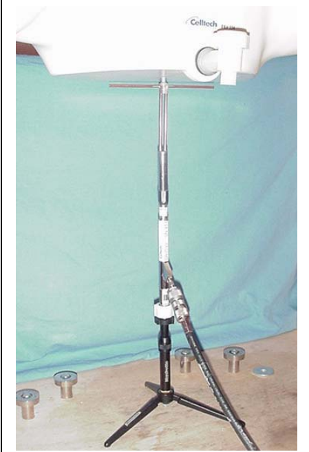
System Performance Check Measurement Setup (IEEE 1528-2003) 835 MHz Validation Dipole Setup
