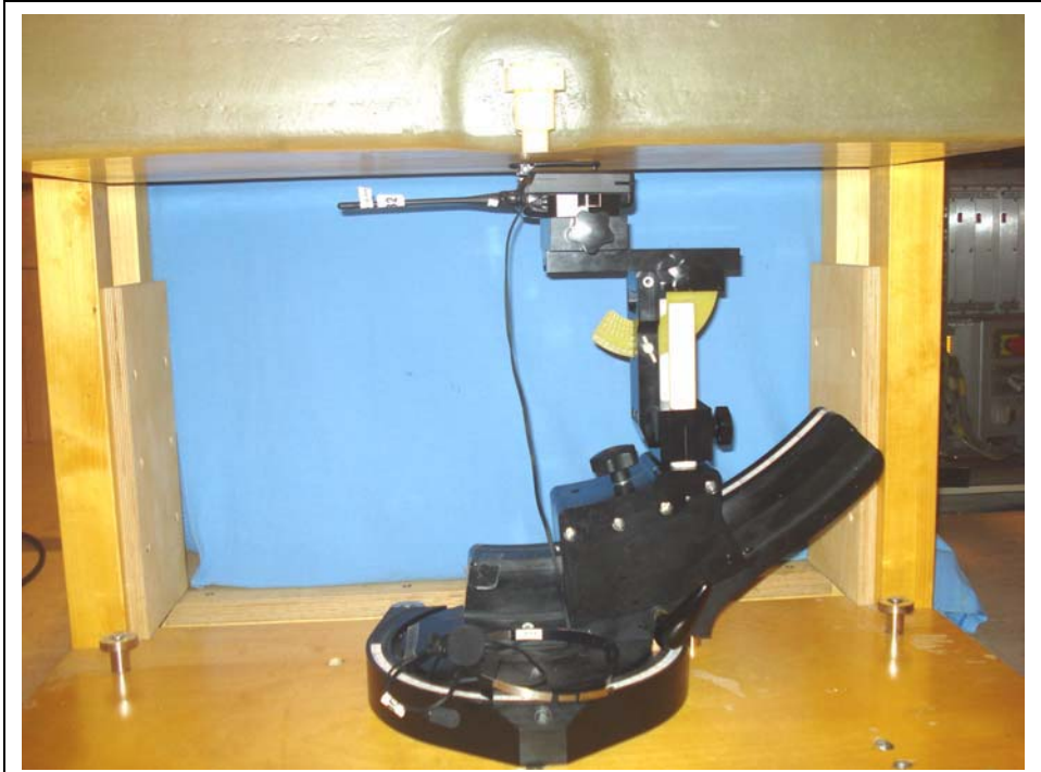
DUT with Headset Boom-Microphone Audio Accessory (P/N: KHS-21)
