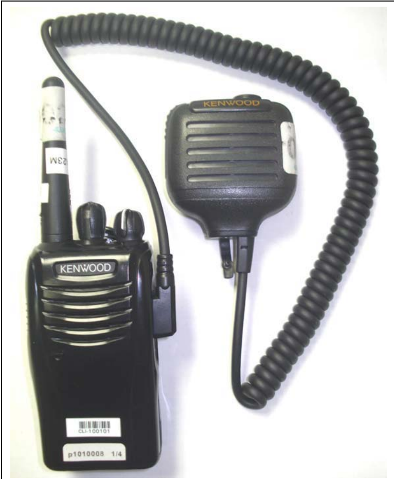
DUT with Speaker-Microphone Audio Accessory P/N: KMC-17
