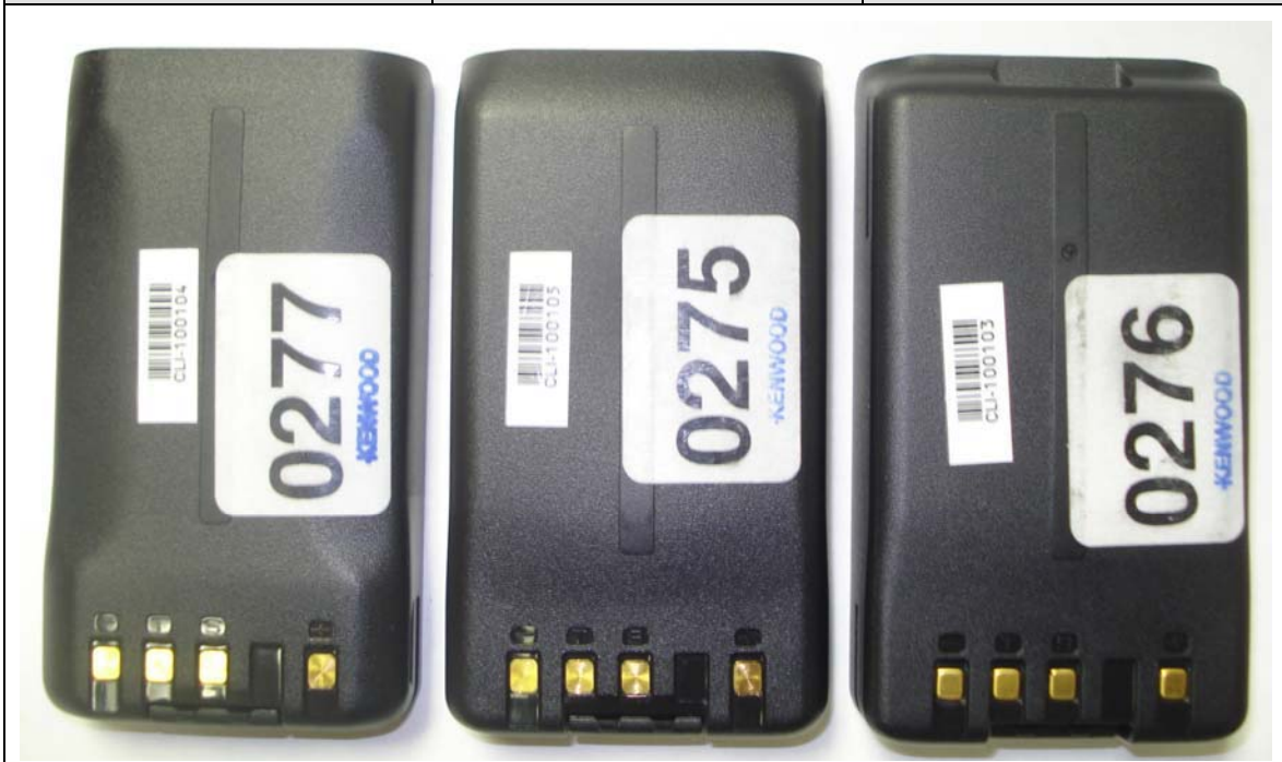
Li-ion Battery P/N: KNB-55L Li-ion Battery P/N: KNB-57L Ni-MH Battery P/N: KNB-56N
