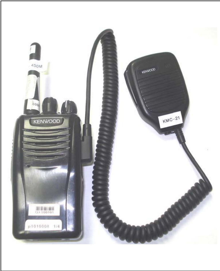
DUT with Speaker-Microphone Audio Accessory P/N: KMC-21
