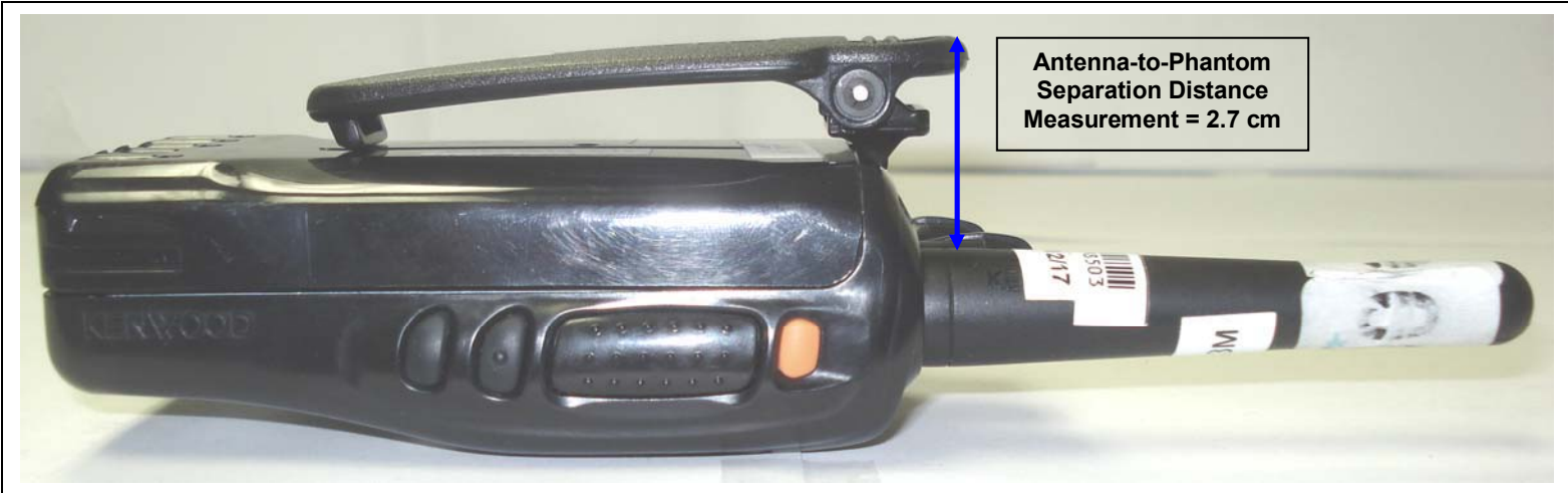
DUT with KNB-55L Li-ion Battery and KRA-23M/M3 Stub Antenna
