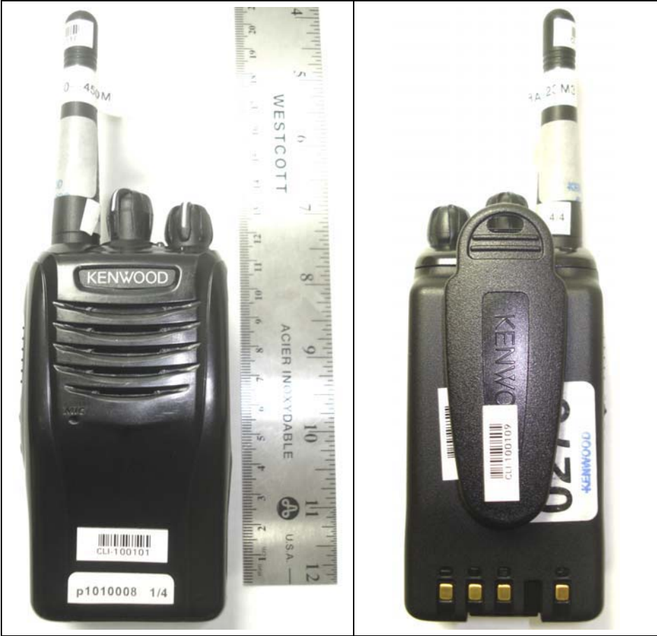
Front of DUT with KRA-23M3 Antenna
