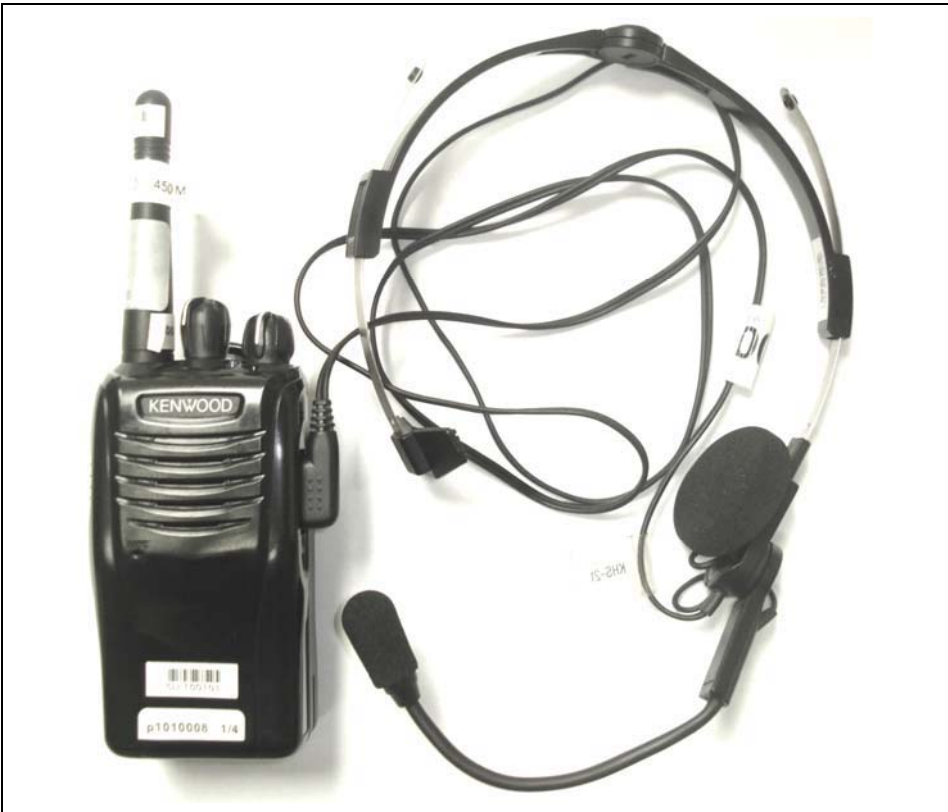
DUT with Headset Boom-Microphone Audio Accessory P/N: KHS-21
