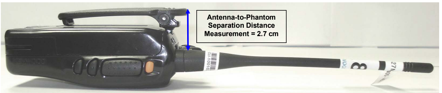
DUT with KNB-57L Li-ion Battery and KRA-27M3 Whip Antenna
