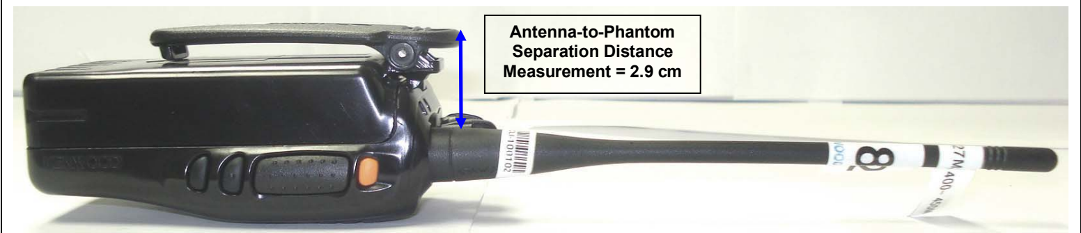
DUT with KNB-56N Ni-MH Battery and KRA-27M3 Whip Antenna
