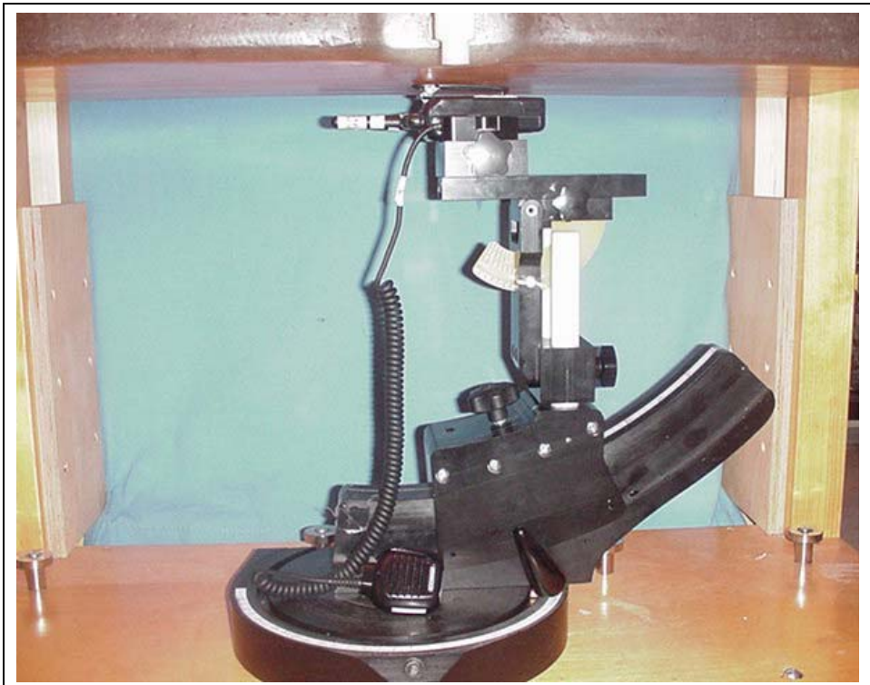
DUT with Speaker-Microphone Audio Accessory (P/N: KMC-45)
