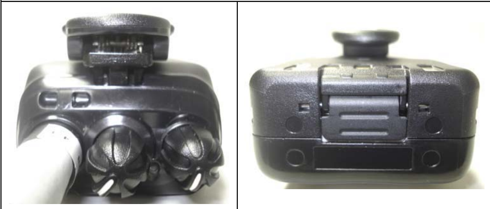
Top and Bottom end of DUT with Li-ion Battery P/N: KNB-57L (2000 mAh)
