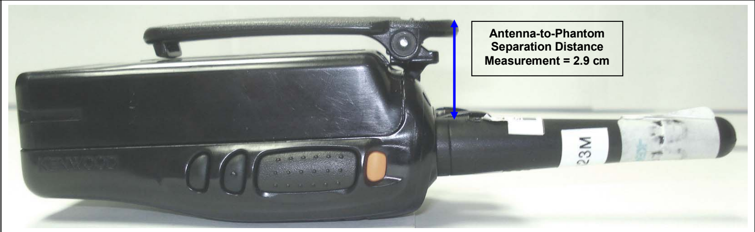
DUT with KNB-56N Ni-MH Battery and KRA-23M/M3 Stub Antenna
