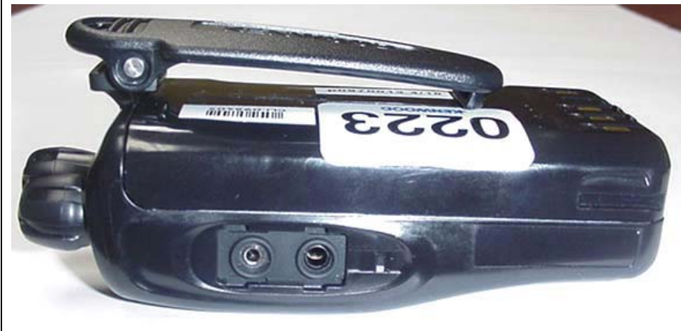
Left and Right Sides of DUT with Li-ion Battery P/N: KNB-55L (1480 mAh)
