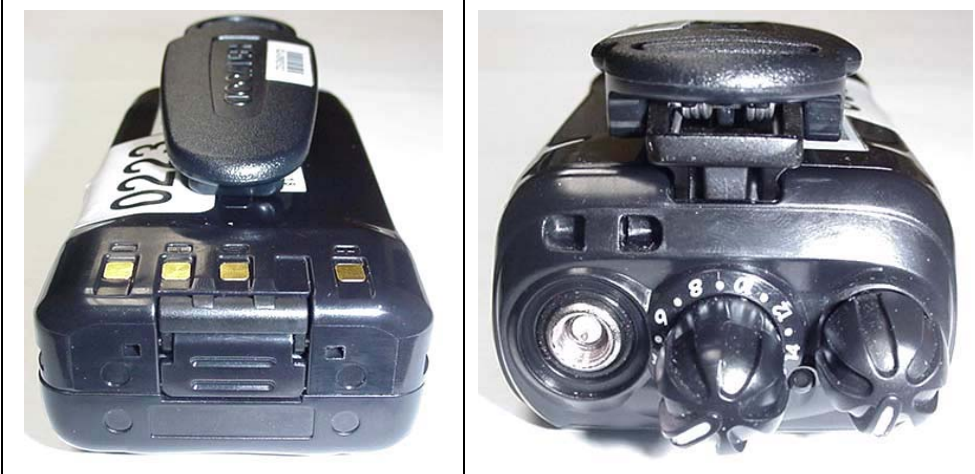
Top and Bottom end of DUT with Li-ion Battery P/N: KNB-55L (1480 mAh)
