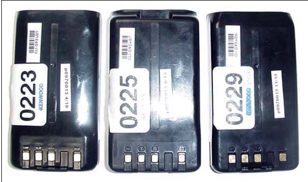
Li-ion Battery P/N: KNB-55L Ni-MH Battery P/N: KNB-56N Li-ion Battery P/N: KNB-57L
