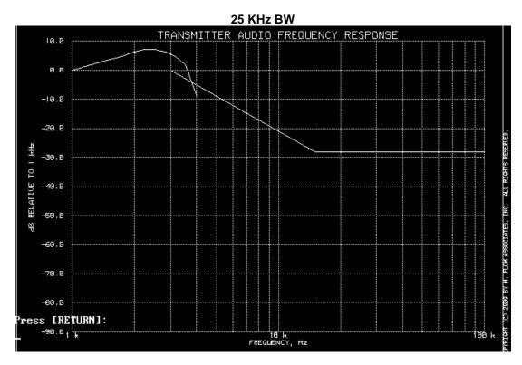
This unit is a digital radio and the roll-off for the filter is very linear in the operational band and sharp out of the band.
