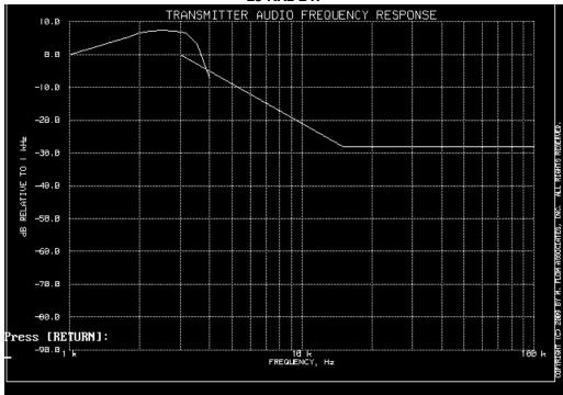
This unit is a digital radio and the roll-off for the filter is very sharp out of the band,
