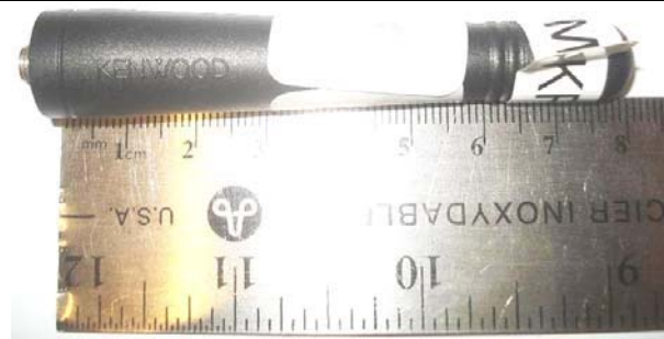
Antenna P/N: KRA-23M3 (Length = 80 mm)
