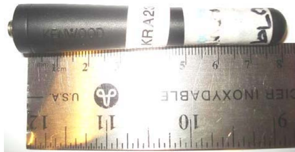
Antenna P/N: KRA-23M (Length = 80 mm)
