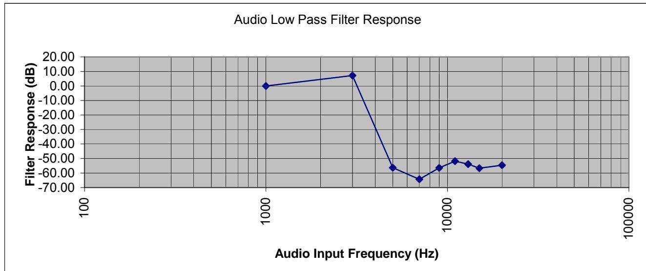
This unit is a digital radio and the roll-off for the filter is very linear in the operational band and sharp out of the band
