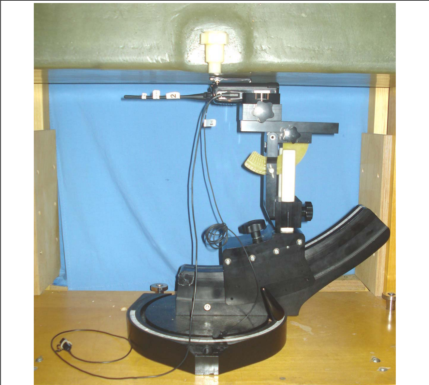
DUT with Belt-Clip Body-worn Accessory (P/N: KBH-10) & Category 2 Default Audio Accessory 2-Wire Ear-Bud w/ mic/PTT (P/N: KHS-23)
