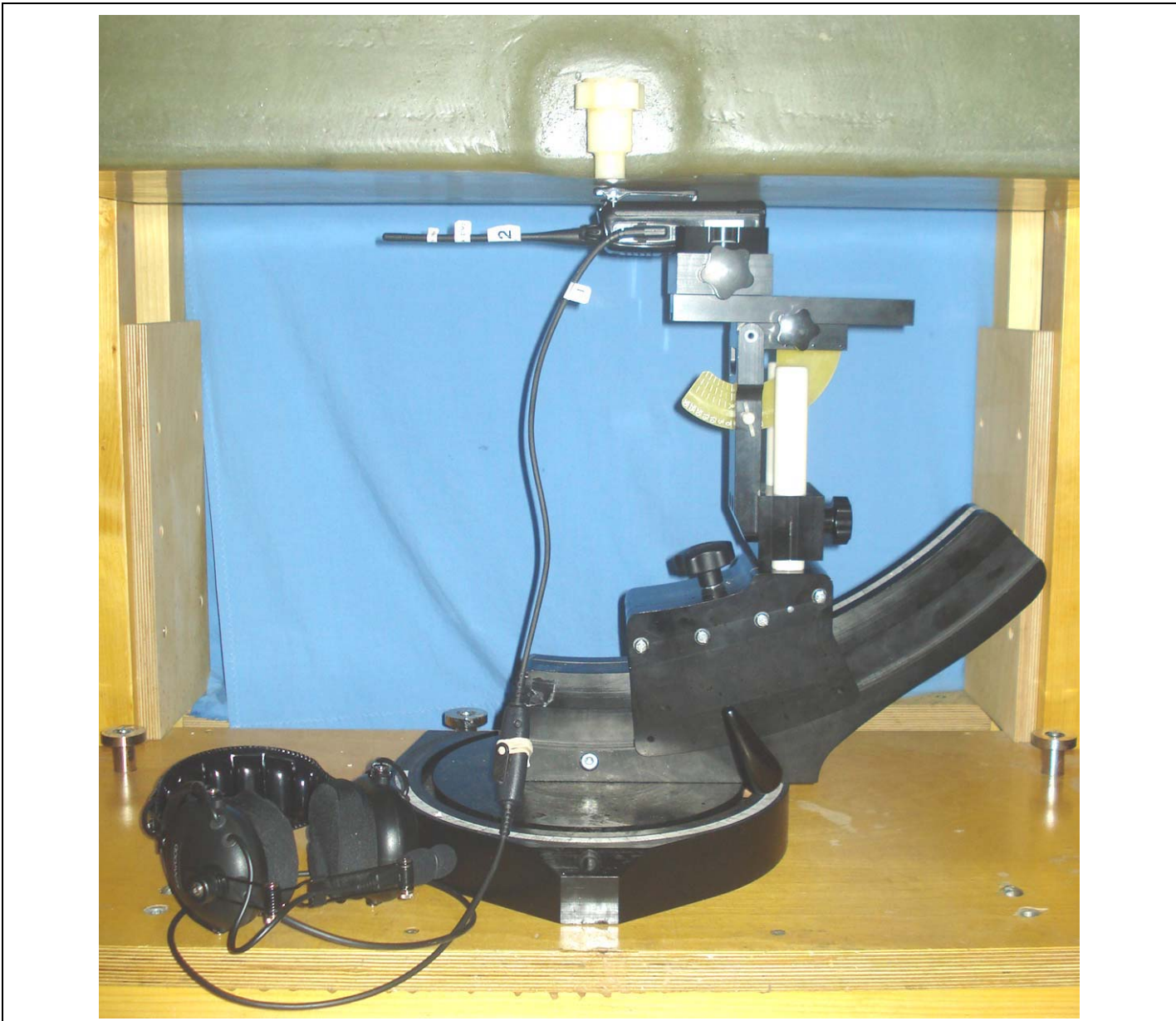
DUT with Belt-Clip Body-worn Accessory (P/N: KBH-10) & Category 1 Default Audio Accessory Over-the-Head Headset (P/N: KHS-10-OH)
