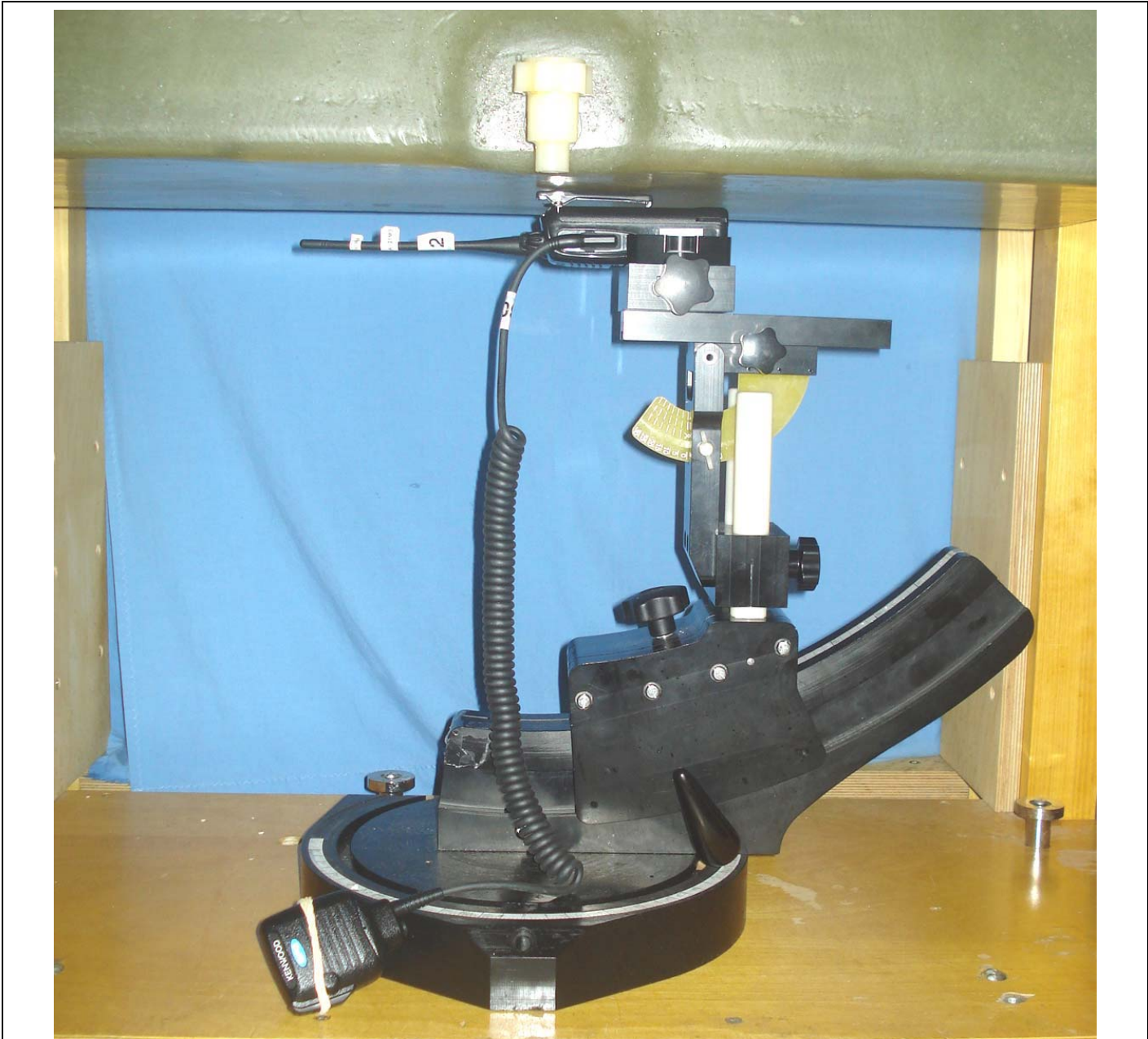
DUT with Belt-Clip Body-worn Accessory (P/N: KBH-10) & Category 4 Default Audio Accessory Speaker-Microphone (P/N: KMC-48GPS)
