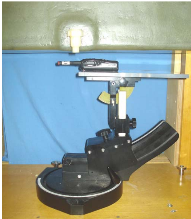
Face-held SAR Test Setup Configuration with Stub Antenna
