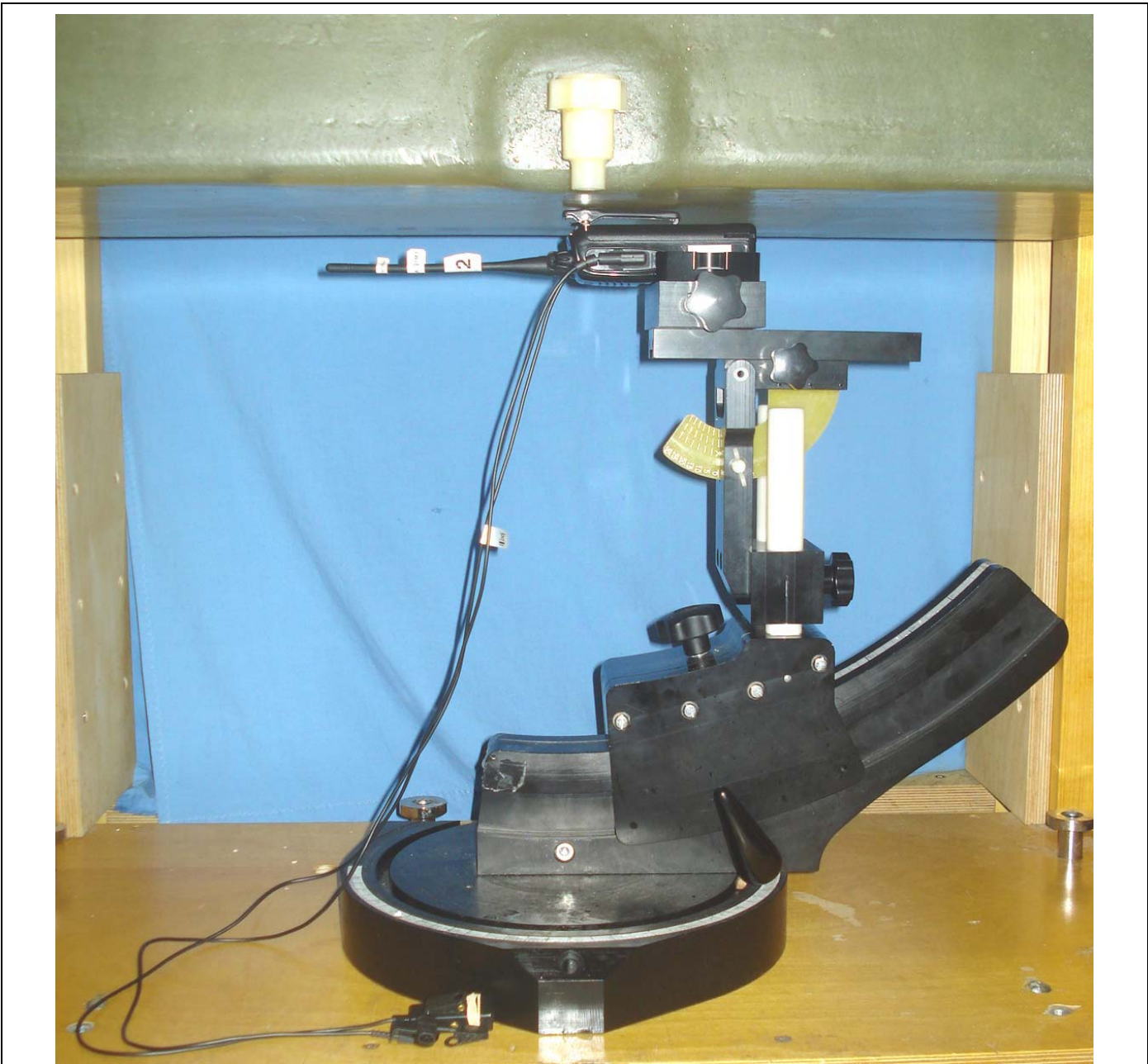
DUT with Belt-Clip Body-worn Accessory (P/N: KBH-10) & Category 3 Default Audio Accessory 2-Wire Palm-Mic Kit (P/N: KHS-8BL)
