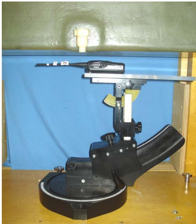
Face-held SAR Test Setup Configuration with Whip Antenna
