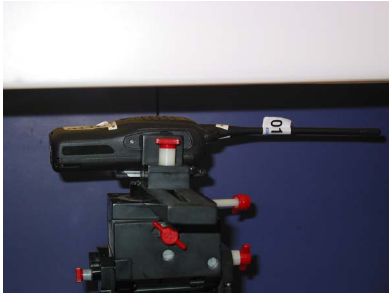
Held to Face Test Position 2.5 cm Gap
