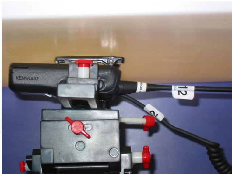
Body Test Position 0 cm Gap
