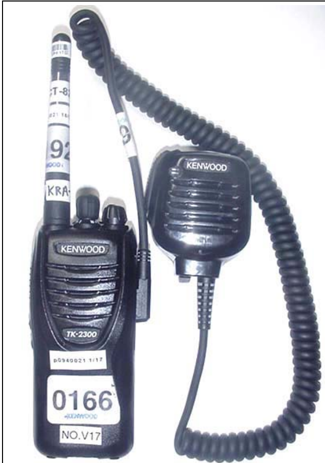
DUT with Speaker-Microphone Audio Accessory (P/N: KMC-45)
