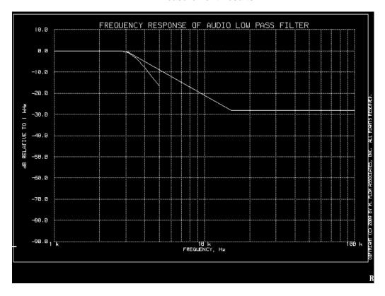
This unit is a digital radio and the roll-off for the filter is very linear in the operational band and sharp out of the band.
