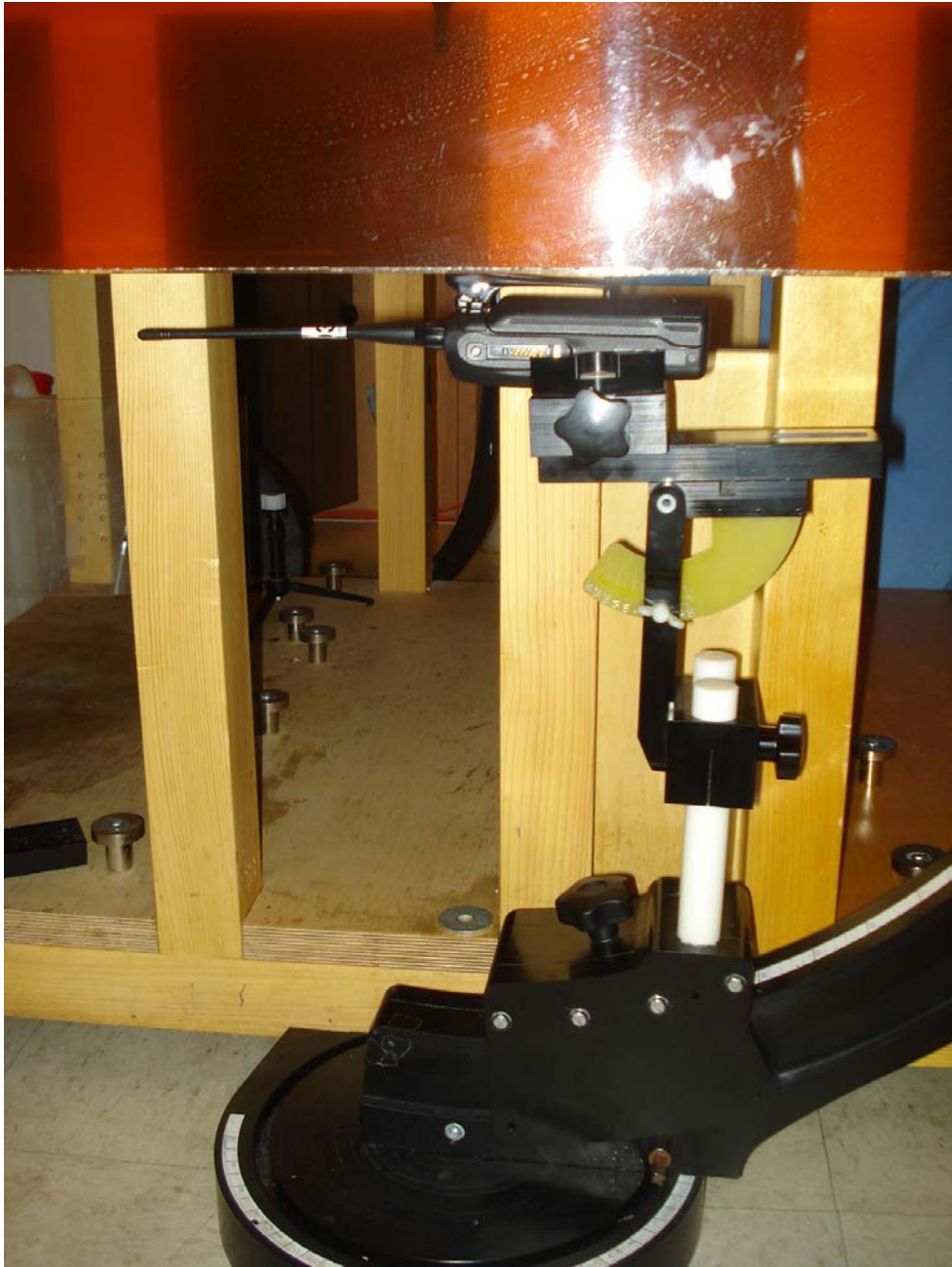
Preliminary Area Scan evaluation – Side Planar Phantom
