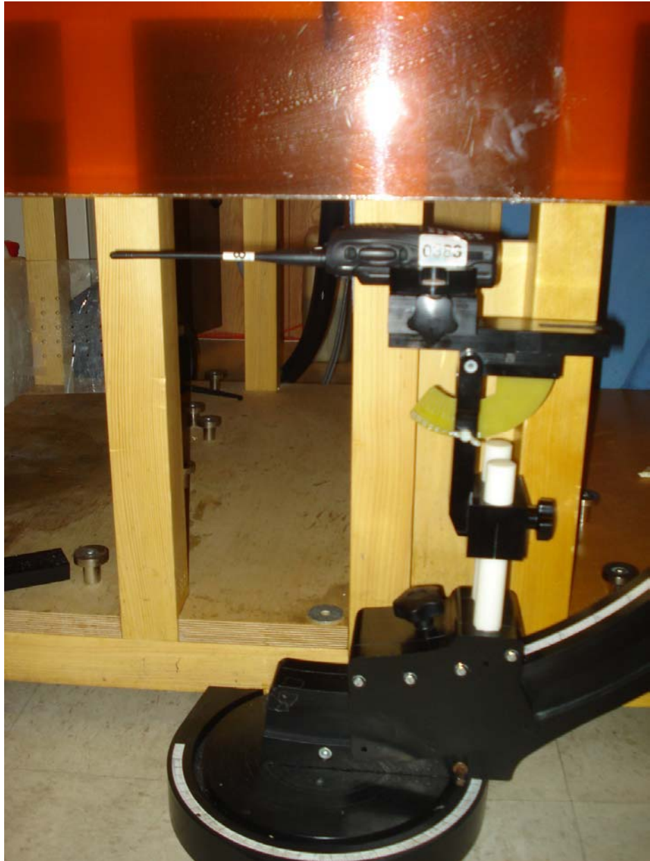
Preliminary Area Scan evaluation – Side Planar Phantom
