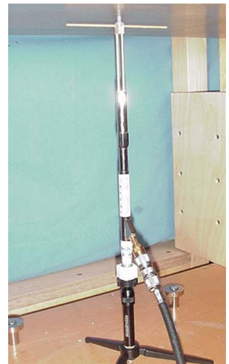
835 MHz SPEAG Validation Dipole Setup
