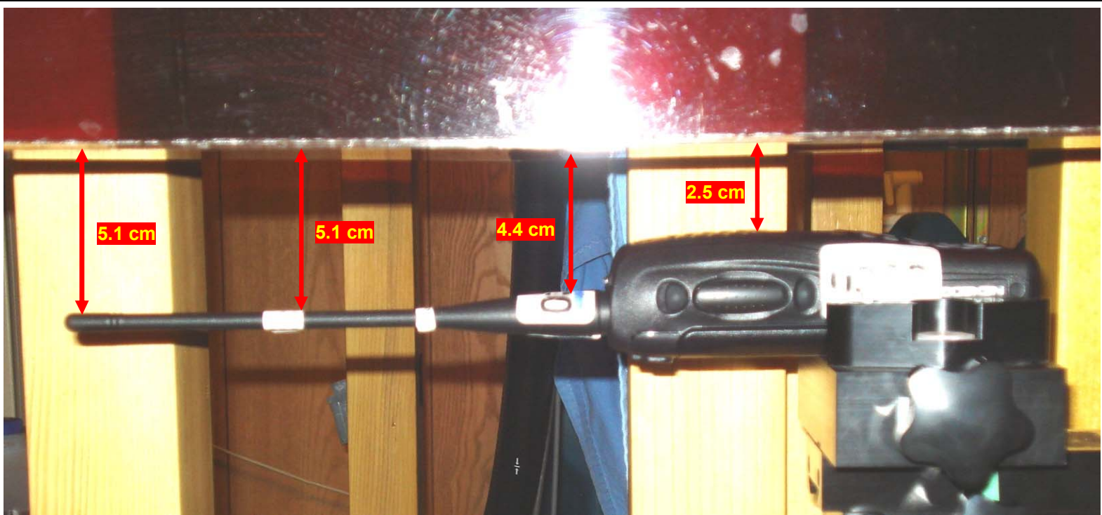
ANTENNA A - Face-held Test Setup with KRA-32 Whip Antenna & Li-Ion Battery "a"
