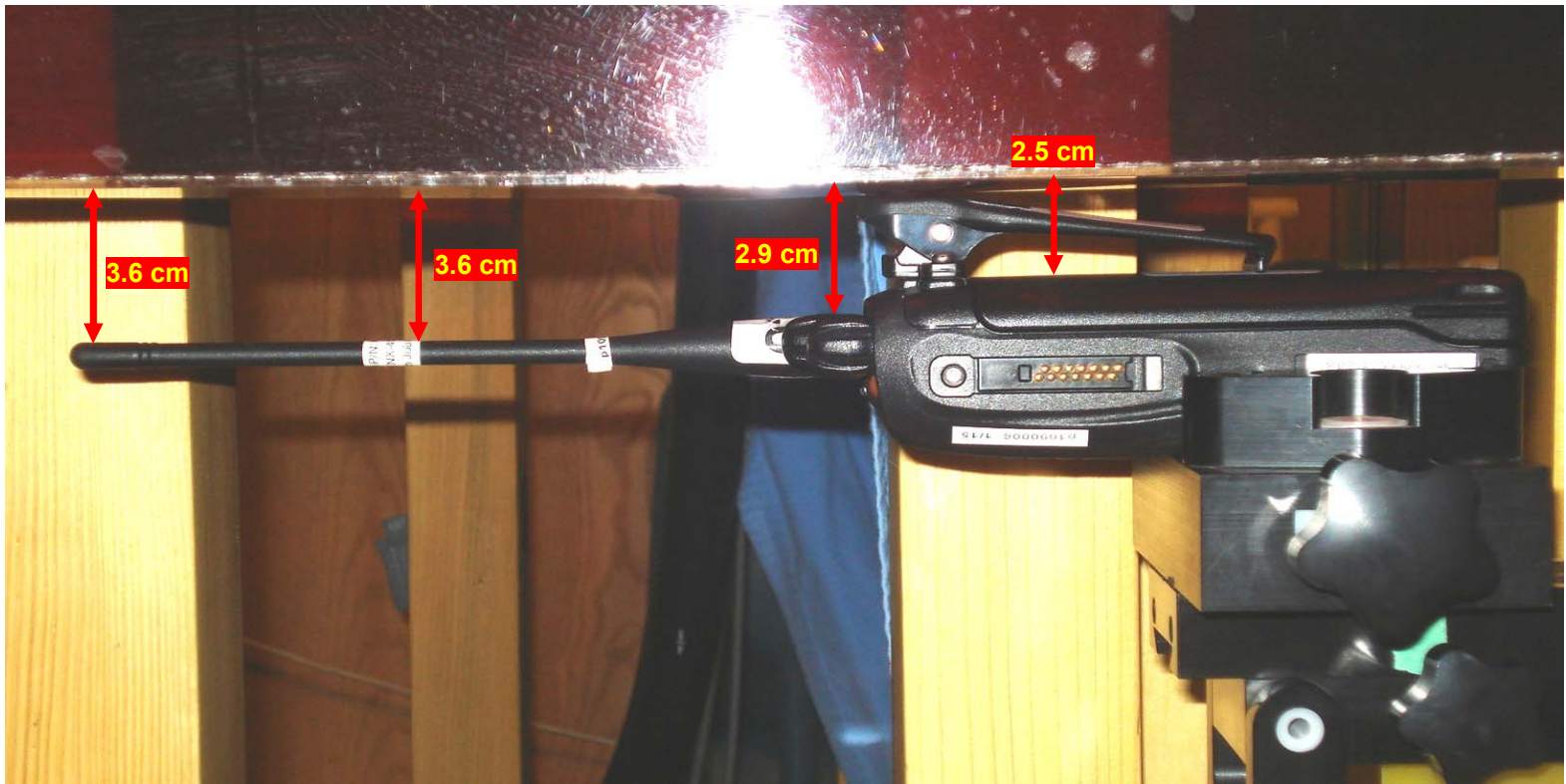
ANTENNA A - Body-worn Test Setup with KRA-32 Whip Antenna & Li-Ion Batt "a" – 2.5 cm Belt-Clip Spacing - Battery Housing Parallel to Planar Phantom
