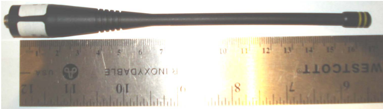
ANTENNA B - Whip Antenna P/N: KRA-24M (Length = 167 mm)
