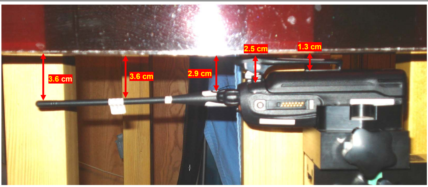
ANTENNA A - Body-worn Test Setup with KRA-32 Whip Antenna & Ni-MH Batt "b" – 2.5 cm Belt-Clip Spacing - Battery Housing Parallel to Phantom
