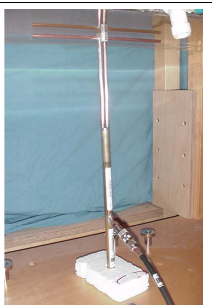
450 MHz Validation Dipole Setup
