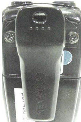
Plastic Belt-Clip with Metal Spring (P/N: J29-0736-XX)
