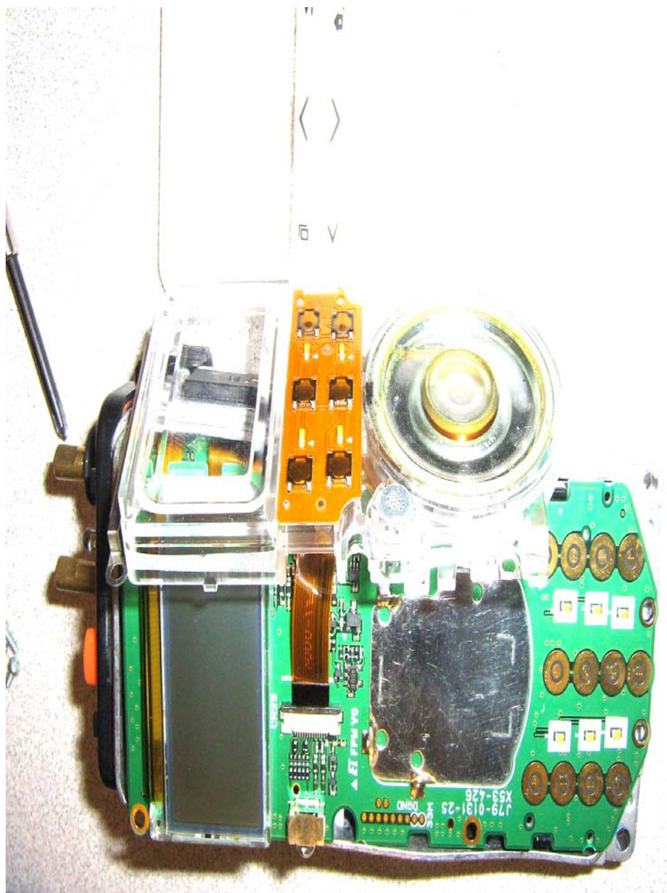
Figure 4 Opened Close Up Switches & LCD
