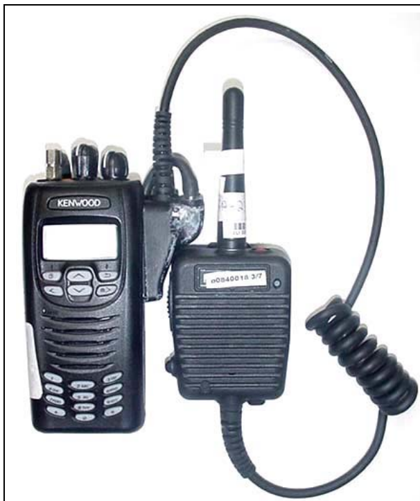
DUT and Speaker-Microphone with KRA-23M Antenna
