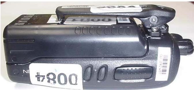
Left Side of Radio with Belt-Clip & Ni-MH Battery (P/N: KNB-50NC)
