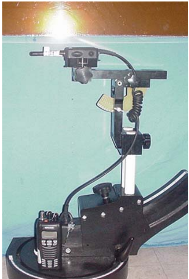
Speaker-Microphone-Antenna Type with KRA-23M3 Antenna 3.1 cm antenna spacing to planar phantom
