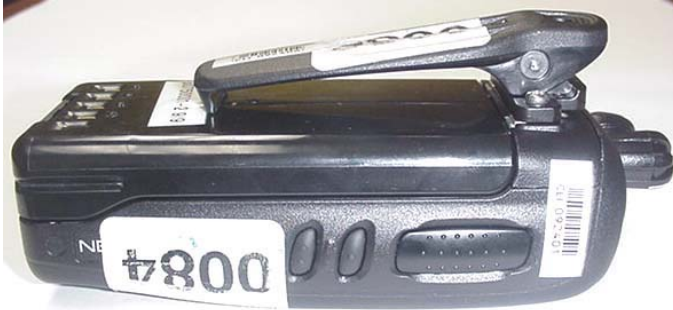
Left Side of Radio with Belt-Clip & Li-ion Battery (P/N: KNB-47L)
