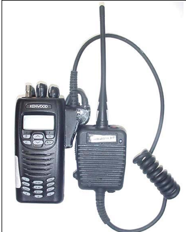
DUT and Speaker-Microphone with KRA-27M Antenna
