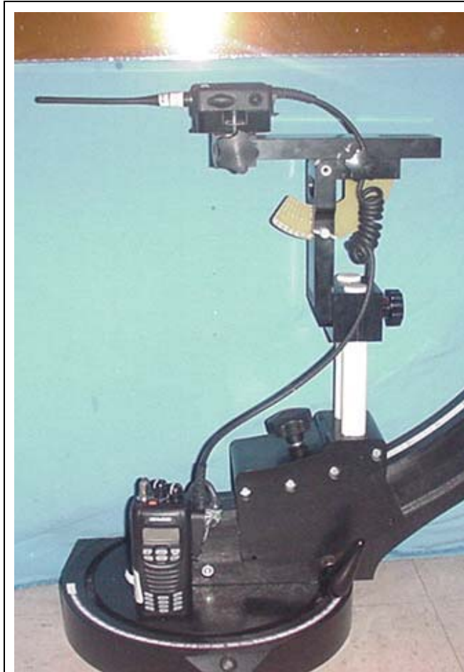
Speaker-Microphone Antenna Type with KRA-27M Antenna 3.1 cm antenna spacing to planar phantom
