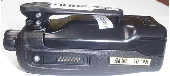
Right Side of Radio with Belt-Clip & Li-ion Battery (P/N: KNB-48L)
