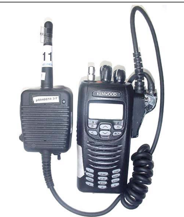
DUT and Speaker-Microphone with KRA-23M3 Antenna
