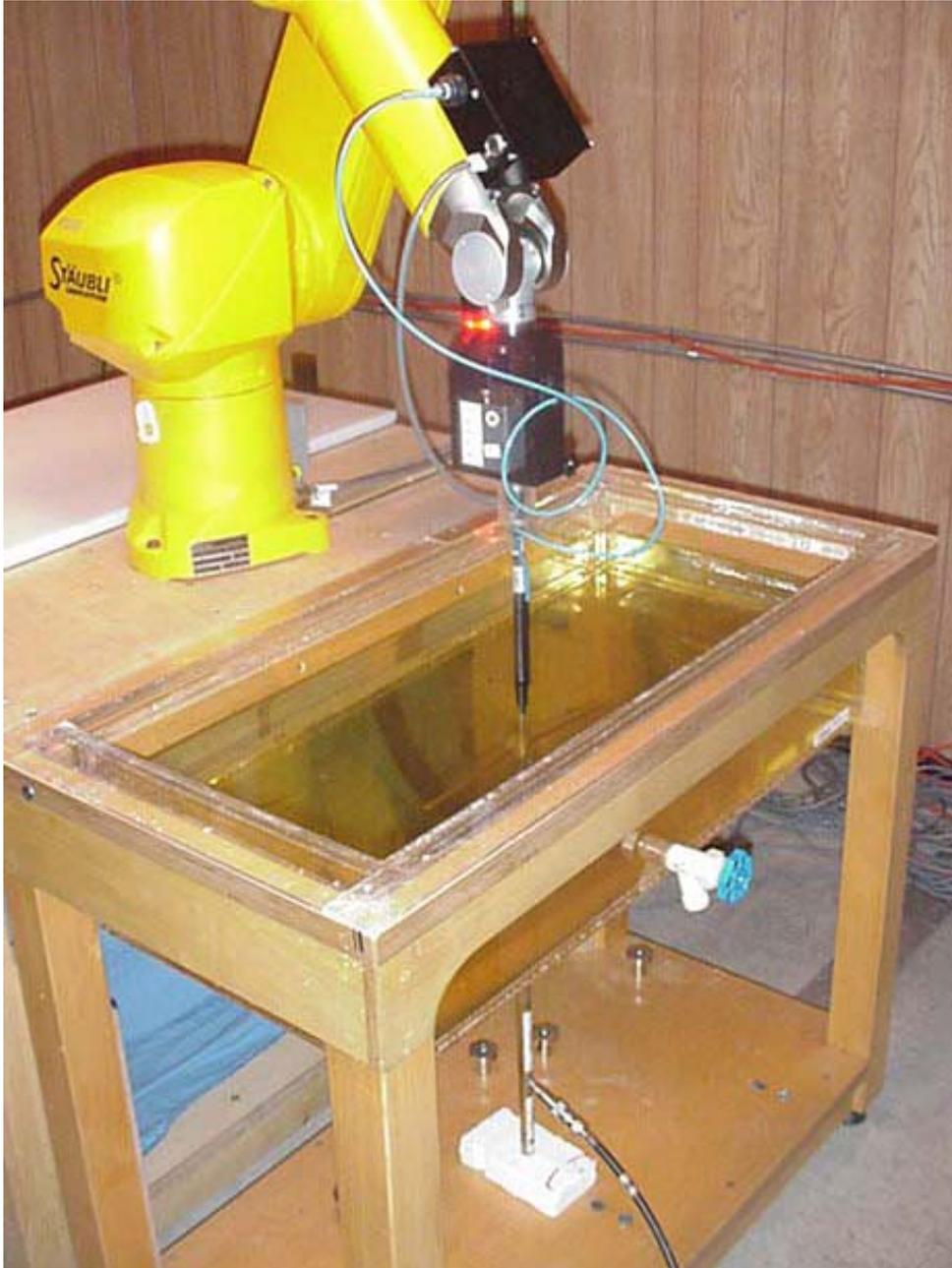
**8. 450 MHz Validation Dipole Setup**
