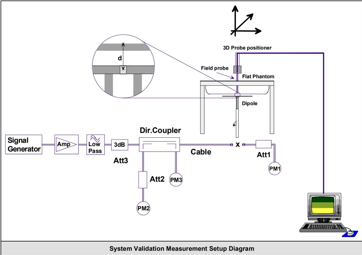
System Validation Measurement Setup Diagram
