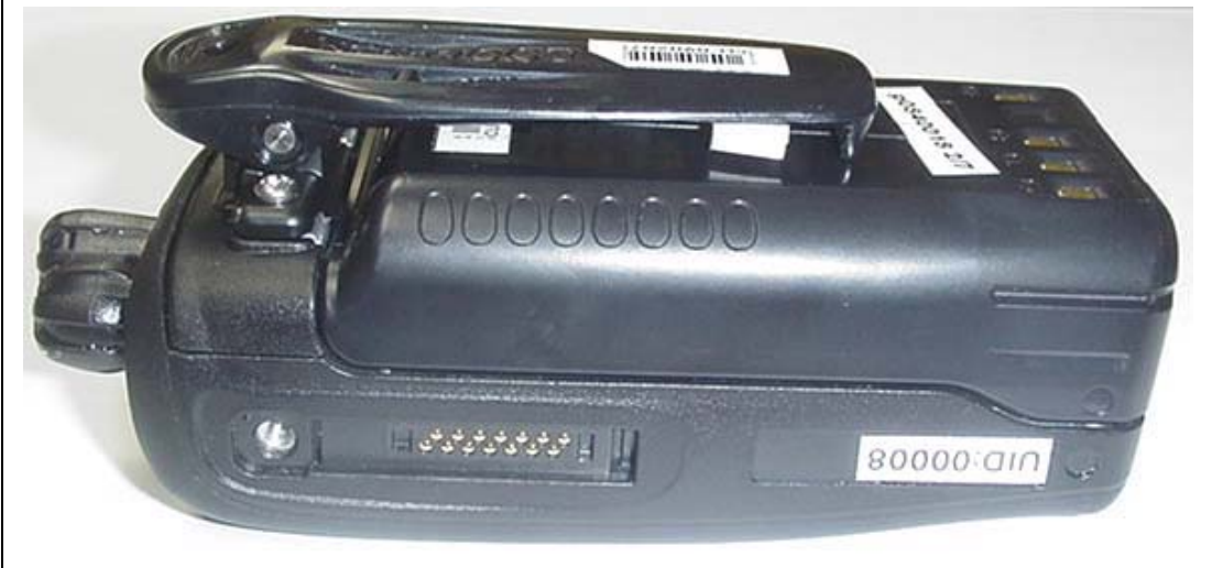
Right Side of Radio Transceiver with Belt-Clip (P/N: J29-0730>PC<1) and Ni-MH Battery (P/N: KNB-50NC)
