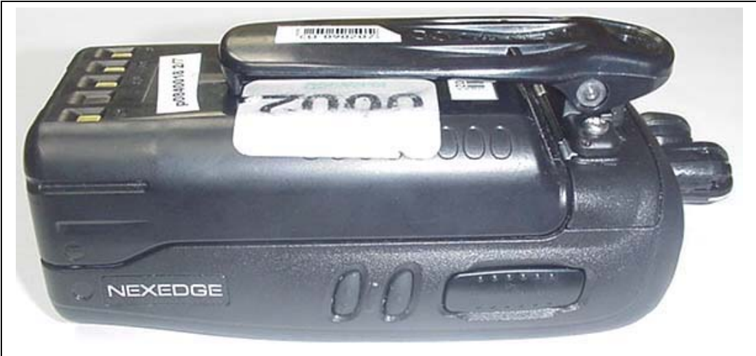
Left Side of Radio Transceiver with Belt-Clip (P/N: J29-0730>PC<1) and Ni-MH Battery (P/N: KNB-50NC)
