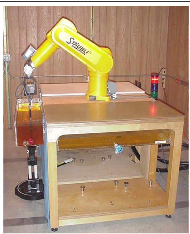
DASY4 SAR Measurement System with Plexiglas side planar phantom
