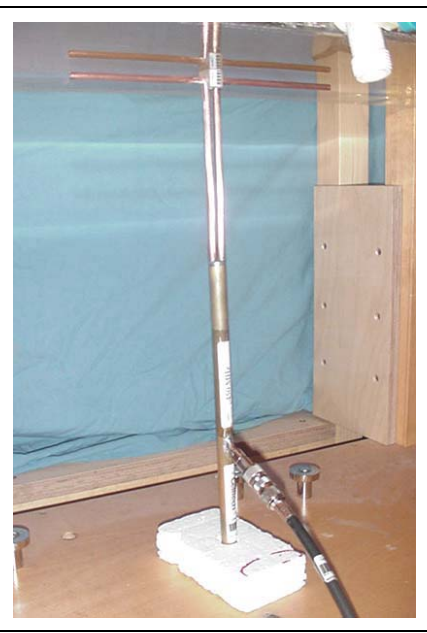
450 MHz Validation Dipole Setup
