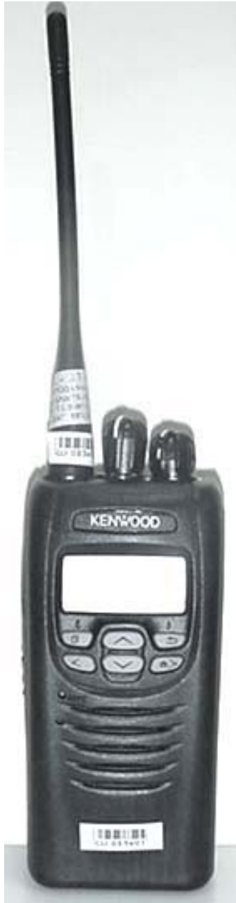
Front of DUT with Whip Antenna (P/N: KRA-27M)
