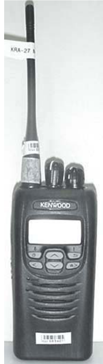
Front of DUT with Whip Antenna (P/N: KRA-27M2)
