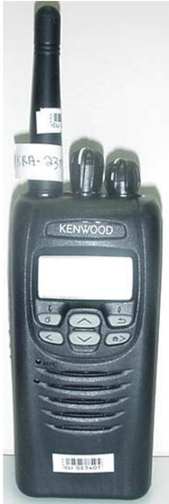
Front of DUT with Helical Antenna (P/N: KRA-23M/M2)
