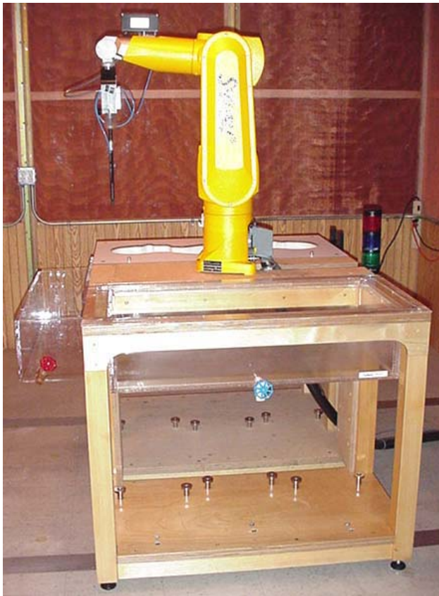
DASY4 SAR Measurement System with validation phantom
