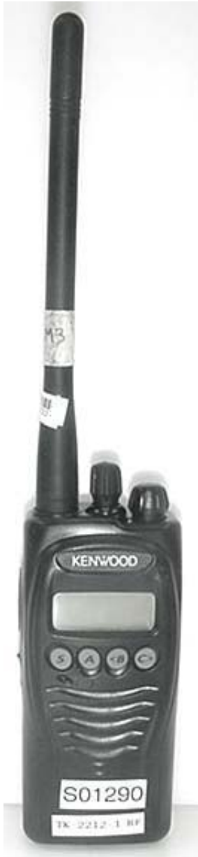
Front of DUT Whip Antenna (P/N: KRA-26M/M2/M3)
