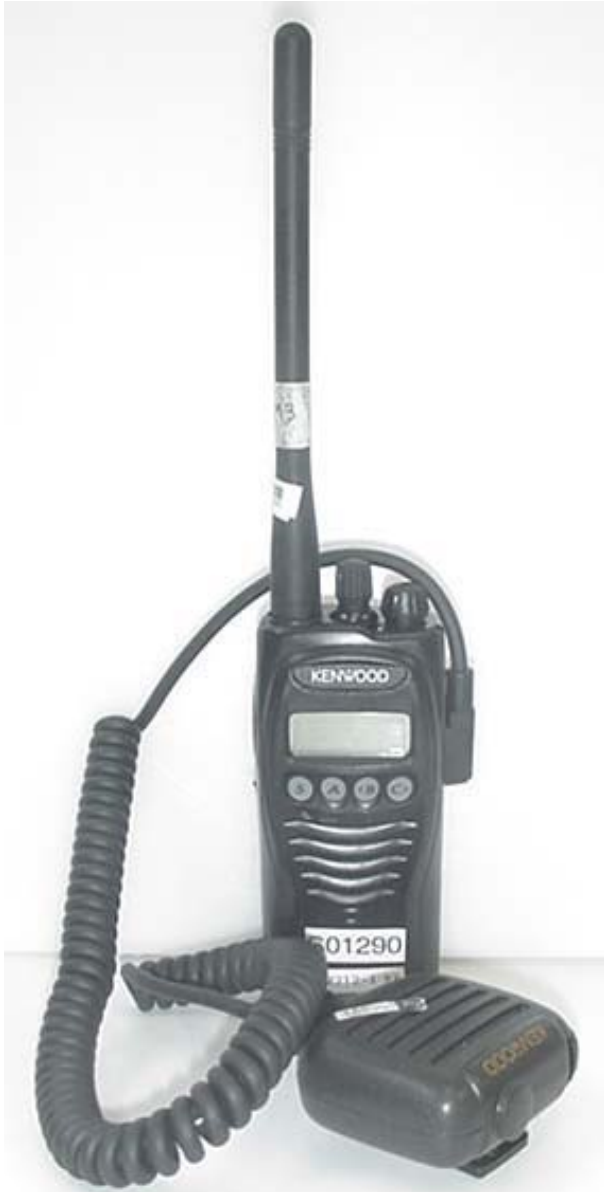
DUT with Speaker-Microphone Accessory (P/N: KMC-17)
