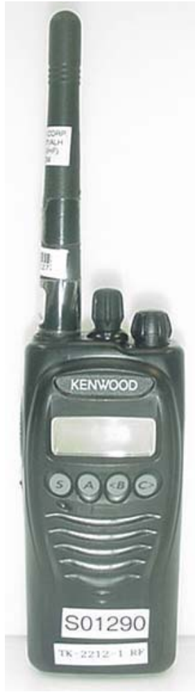
Front of DUT Stubby Antenna (P/N: KRA-22M/M2/M3)
