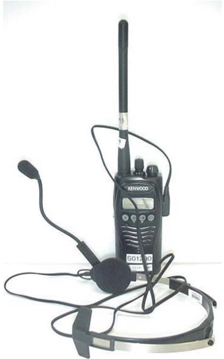
DUT with Boom-Microphone Headset Accessory (P/N: KHS-21)
