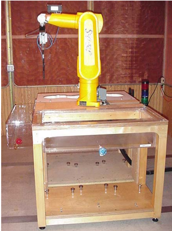
DASY4 SAR Measurement System with validation phantom
