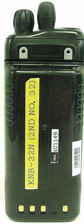
Back of DUT with NiMH Battery
