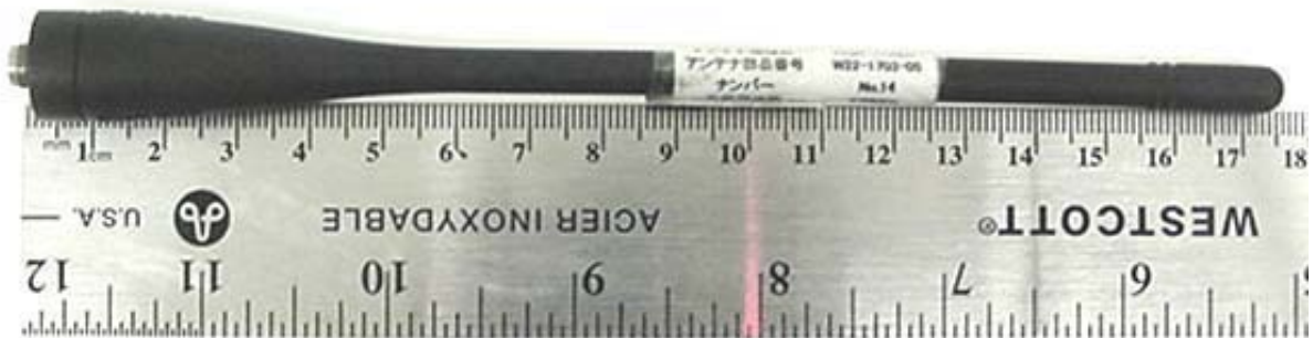
Whip Antenna (P/N: KRA-27M3)
