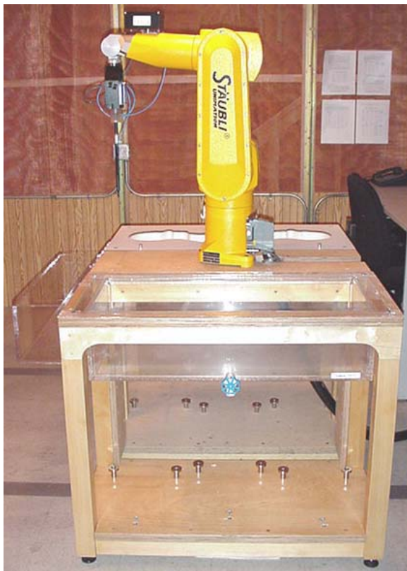
DASY4 SAR Measurement System with validation phantom
