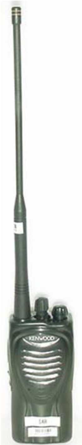
Front of DUT Long Whip Antenna
