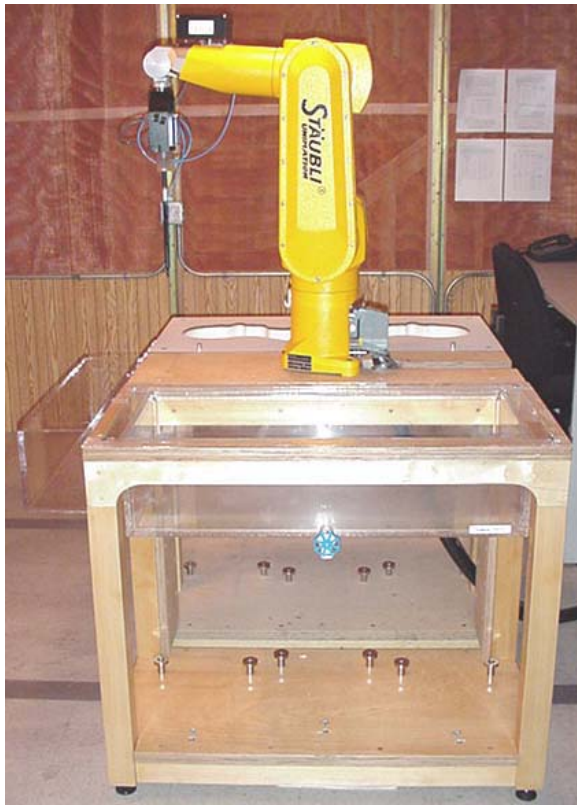
DASY4 SAR Measurement System with validation phantom
