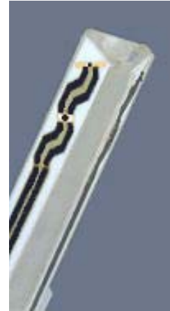
ET3DV6 E-Field Probe
