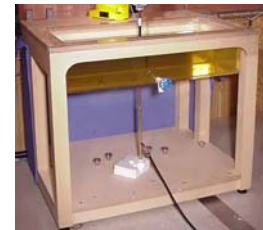
Validation Planar Phantom
