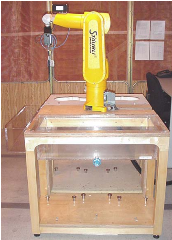
DASY4 SAR Measurement System with validation phantom
