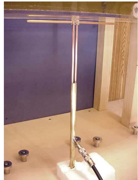
450MHz System Check Setup
