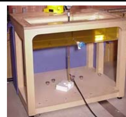
Validation Planar Phantom
