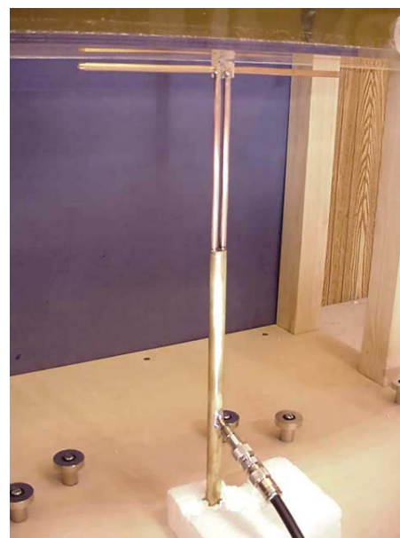
450MHz System Check Setup
