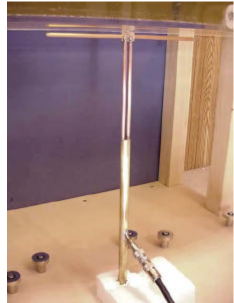
450MHz System Check Setup
