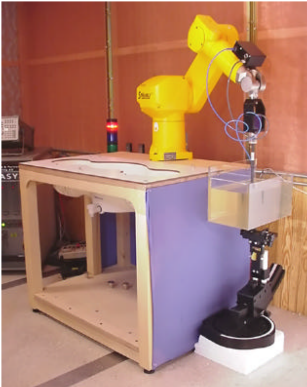
DASY3 SAR Measurement System with Planar Phantom
