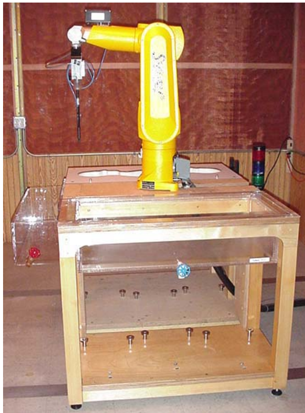
DASY4 SAR Measurement System with validation phantom
