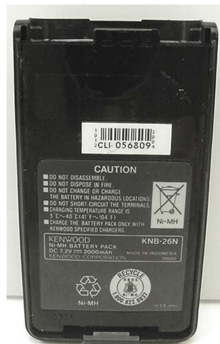
NiMH Battery (P/N: KNB-26N)
