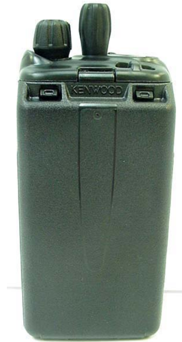
Back of DUT with Alkaline Battery Pack
