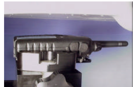
Face-held SAR Test Setup 2.5cm Separation Distance
