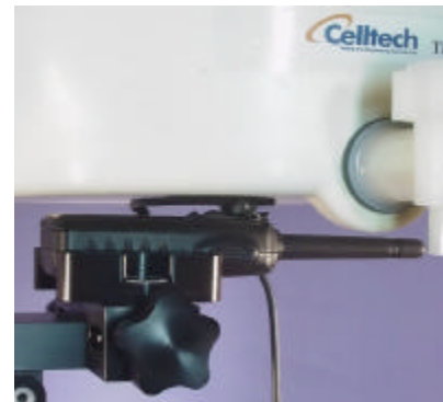
Body-worn SAR Test Setup with 1.0cm Belt-Clip & Speaker-Mic
