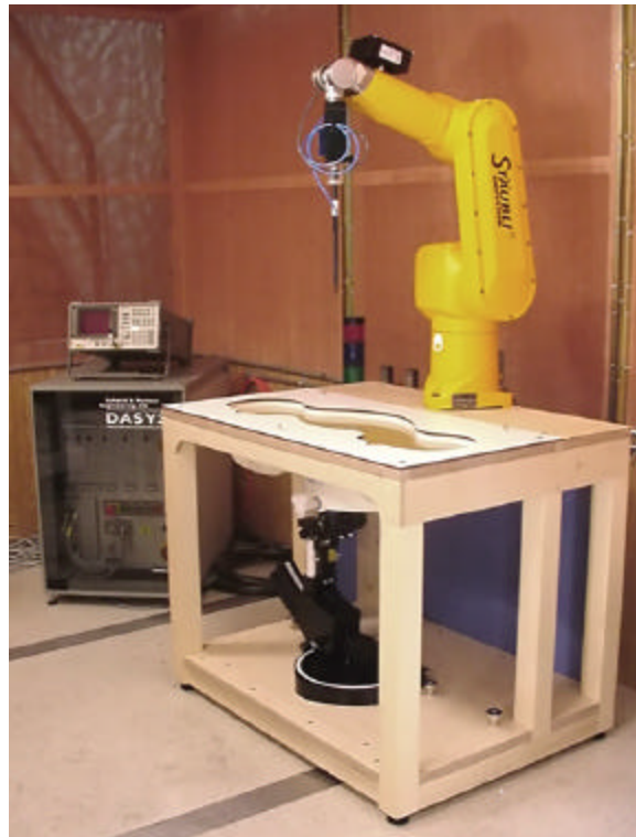
DASY3 SAR Measurement System with SAM phantom
