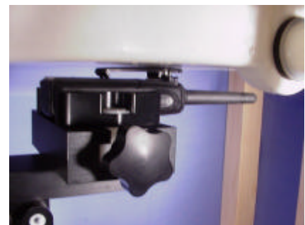
Body-worn SAR Test Setup with 1.0cm Belt-Clip
