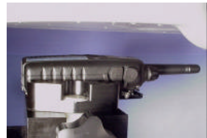
Face-held SAR Test Setup 2.5cm Separation Distance
