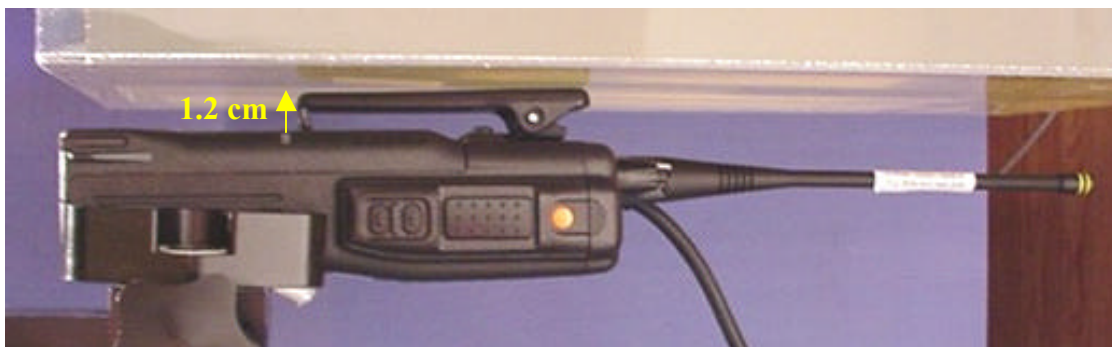
Body-worn SAR Test Setup - 1.2cm Belt-Clip Separation Distance
