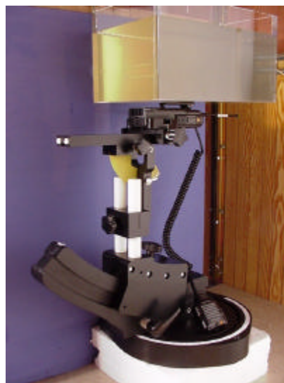
Body-worn SAR Test Setup with small planar phantom
