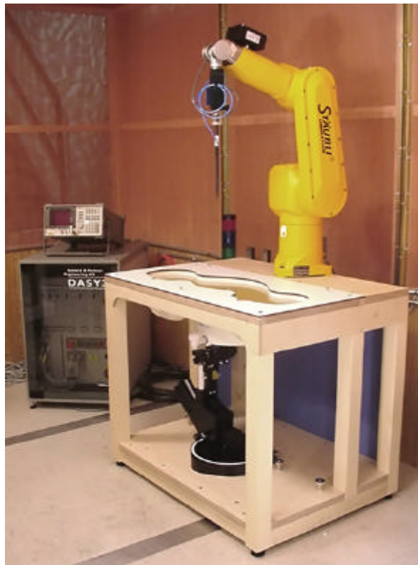
DASY3 SAR Measurement System with SAM phantom
