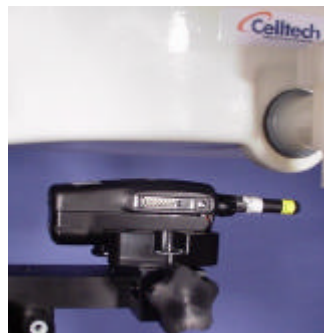
Face-held SAR Test Setup 2.5cm Separation Distance
