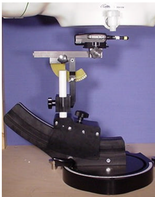
Face SAR Test Setup with SAM Planar Phantom
