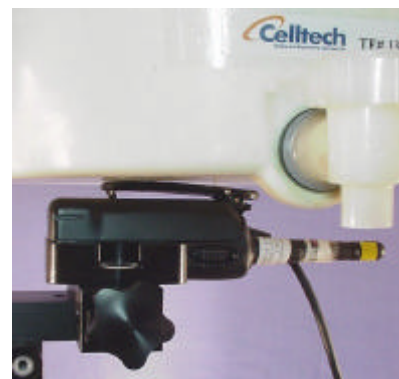
Body-worn SAR Test Setup with Belt-Clip & Speaker-Mic (Belt-Clip providing a 1.0cm Separation)
