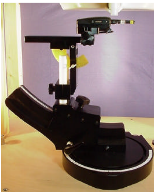
Face SAR Test Setup with SAM Planar Phantom
