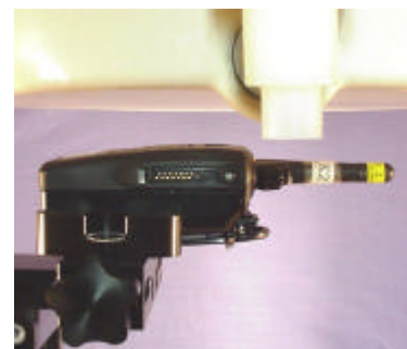
Face-held SAR Test Setup 2.5cm Separation Distance
