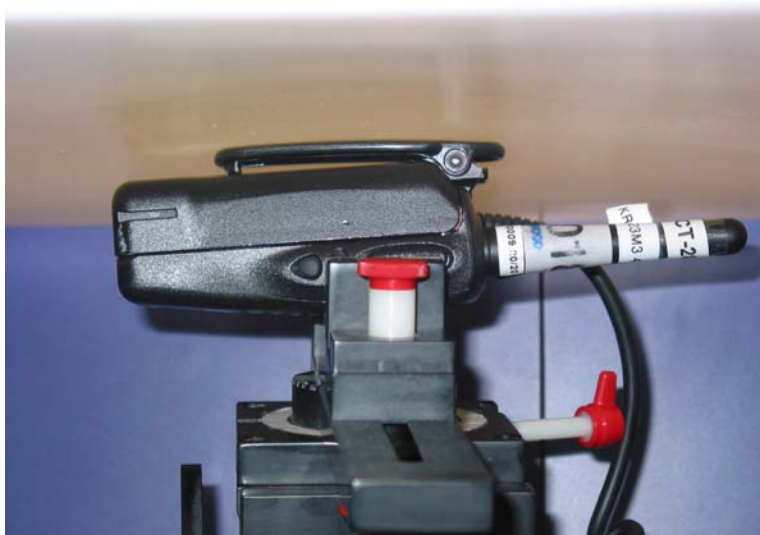
Body Test Position 0 cm Gap
