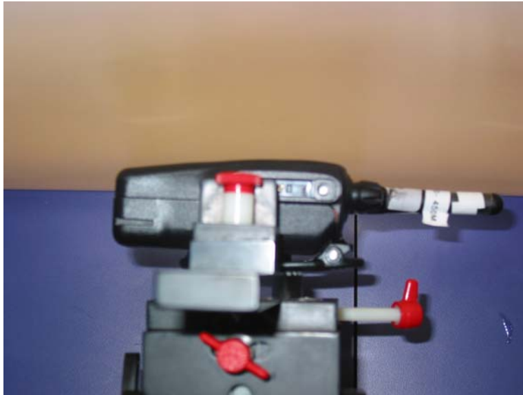
Held to Face Test Position 2.5 cm Gap
