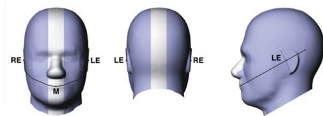
Figure 6.2 Front, back and side view of SAM
