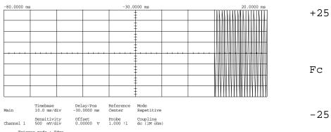
Trigger mode : Edge On Positive Edge Of Chan2 Trigger Level Chan2 = -1.37500 V (noise reject ON) Holdoff = 40.000 ns
