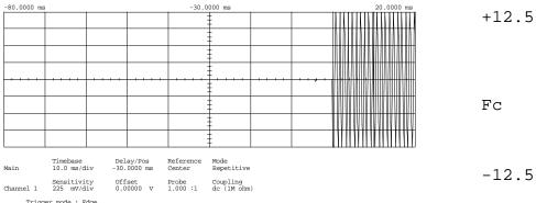
Trigger mode : Edge On Positive Edge Of Chan2 Trigger Level Chan2 = -787.500 mV (noise reject ON) Holdoff = 40.000 ns
