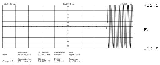
Trigger mode : Edge On Positive Edge Of Chan2 Trigger Level Chan2 = -875.000 mV (noise reject ON) Holdoff = 40.000 ns
