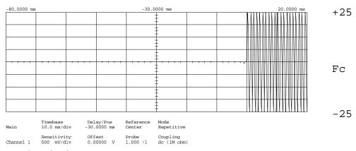
Trigger mode : Edge On Positive Edge Of Chan2 Trigger Level Chan2 = -812.500 mV (noise reject ON) Holdoff = 40.000 ns
