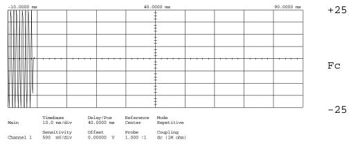
Trigger mode : Edge On Negative Edge Of Chan2 Trigger Level Chan2 = -17.500 mV (noise reject ON) Holdoff = 40.000 ns
