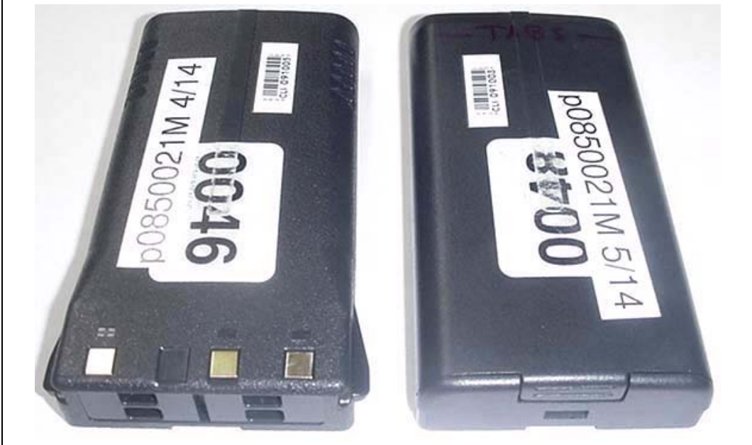
NiMH 7.2V 1600mAh Battery (P/N: KNB-20N) Alkaline AA Battery Case (P/N: KBP-1)
