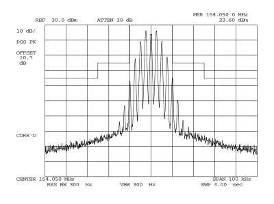
POWER: MODULATION: LOW VOICE: 2500 Hz SINE WAVE MASK: B, VHF/UHF 25kHz, w/LPF
