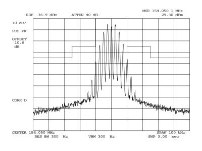
POWER: MODULATION: HIGH VOICE: 2500 Hz SINE WAVE MASK: B, VHF/UHF 25kHz, w/LPF
