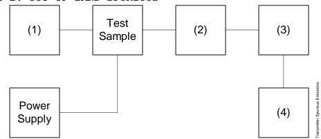
Asset Description s/n (as applicable) (1) AUDIO OSCILLATOR/GENERATOR i00010 HP 204D 1105A04683 i00017 HP 8903A 2216A01753 i00012 HP 3312A 1432A11250 (2) COAXIAL ATTENUATOR i00122 Narda 766-10 7802 i00123 Narda 766-10 7802A i00069 Bird 8329 (30 dB) 1006 i00113 Sierra 661A-3D 1059 (3) FILTERS; NOTCH, HP, LP, BP i00126 Eagle TNF-1 i00125 Eagle TNF-1 100-250 50-60 i00124 Eagle TNF-1 250-850
