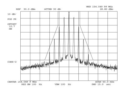
POWER: MODULATION: LOW VOICE: 2500 Hz SINE WAVE MASK: D, VHF/UHF 12.5kHz BW
