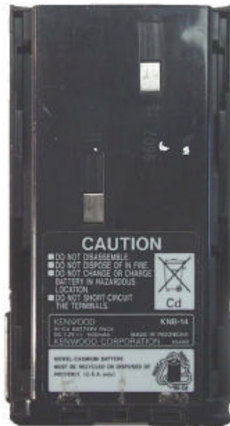
< Ni-Cd Battery (DC 7.2V/600mAh, M/N : KNB-14) >
