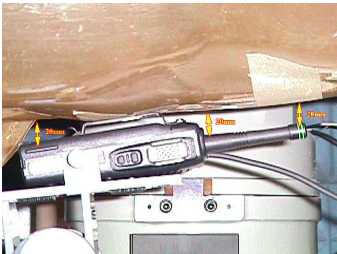
< Close-up view – Waist with the belt-clip and the high capacity battery pack (M/N :KNB-15A) >
