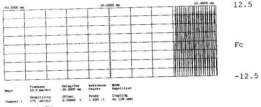
Trigger mode : Edge On Positive Edge Of Chan2 Trigger Level Chan2 = -962.500 mV (noise reject ON) Holdoff = 40.000 ns
