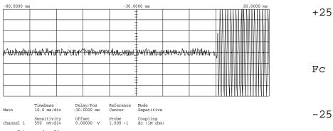
Trigger mode : Edge On Positive Edge Of Chan2 Trigger Level Chan2 = -1.10000 V (noise reject ON) Holdoff = 40.000 ns
