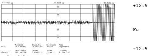
Trigger mode : Edge On Positive Edge Of Chan2 Trigger Level Chan2 = -875.000 mV (noise reject ON) Holdoff = 40.000 ns
