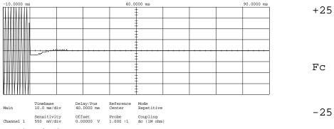
Trigger mode : Edge On Negative Edge Of Chan2 Trigger Level Chan2 = -3.500 mV (noise reject ON) Holdoff = 40.000 ns
