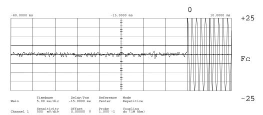
Trigger mode : Edge On Positive Edge Of Chan2 Trigger Level Chan2 = -187.500 mV (noise reject ON) Holdoff = 40.000 ns
