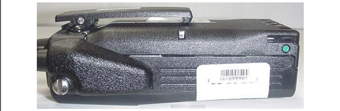
Left & Right Sides of DUT with Ni-Cd IS 1500mAh Battery P/N: KNB-17B & Belt-Clip accessory P/N: KBH-10
