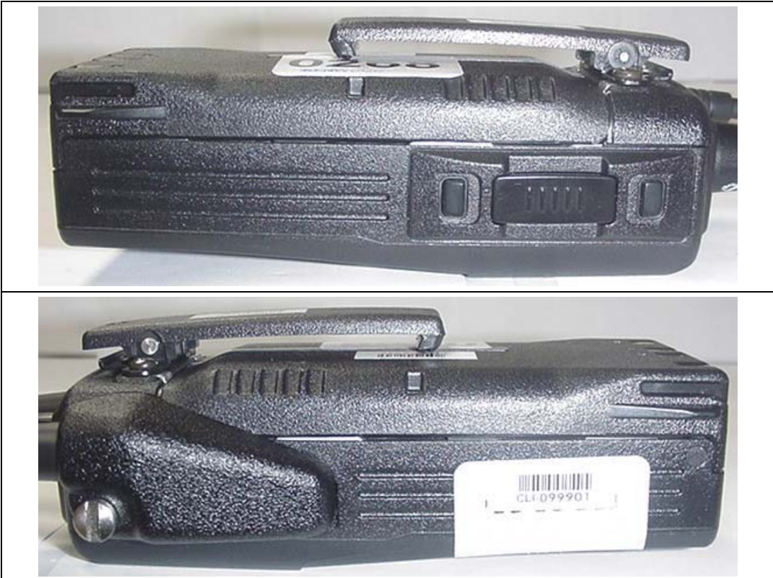
Left & Right Sides of DUT with Ni-MH 2100mAh Battery P/N: KNB-22N & Belt-Clip accessory P/N: KBH-10
