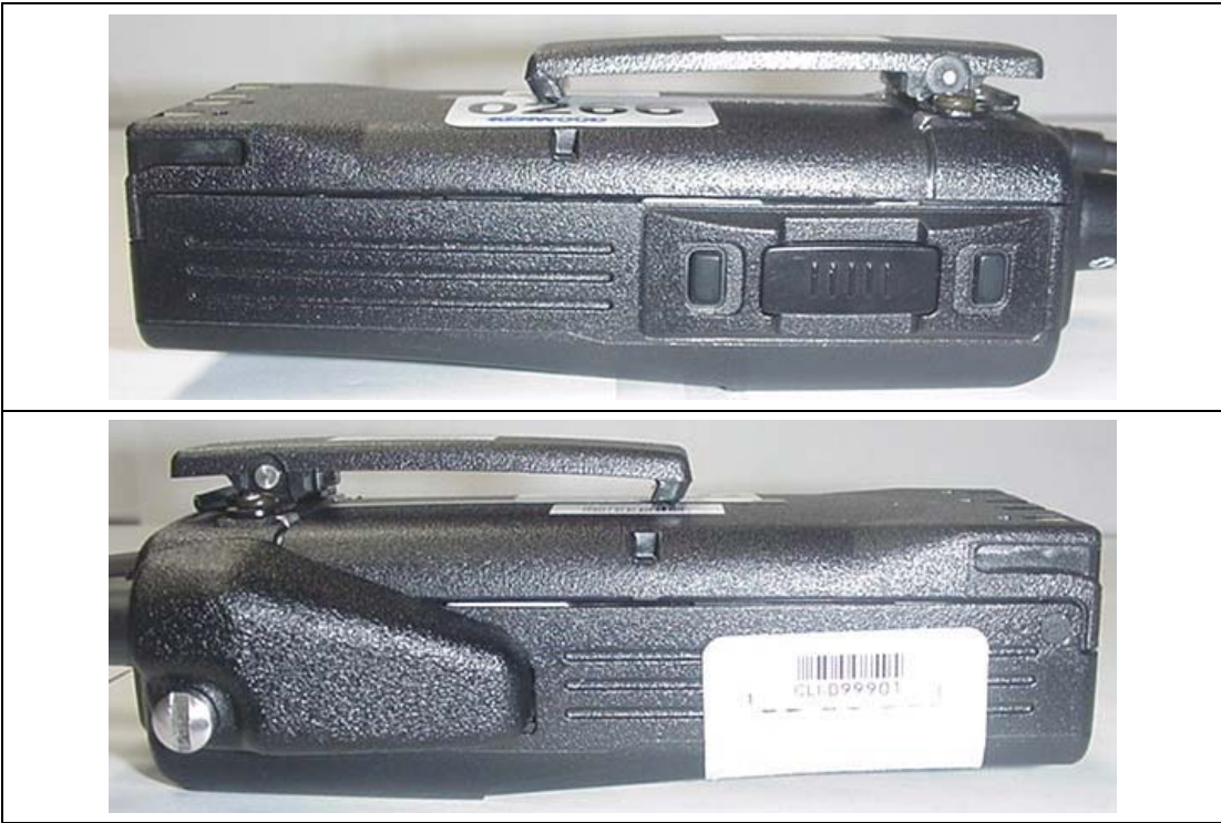
Left & Right Sides of DUT with Ni-MH 1400mAh Battery P/N: KNB-52N & Belt-Clip accessory P/N: KBH-10
