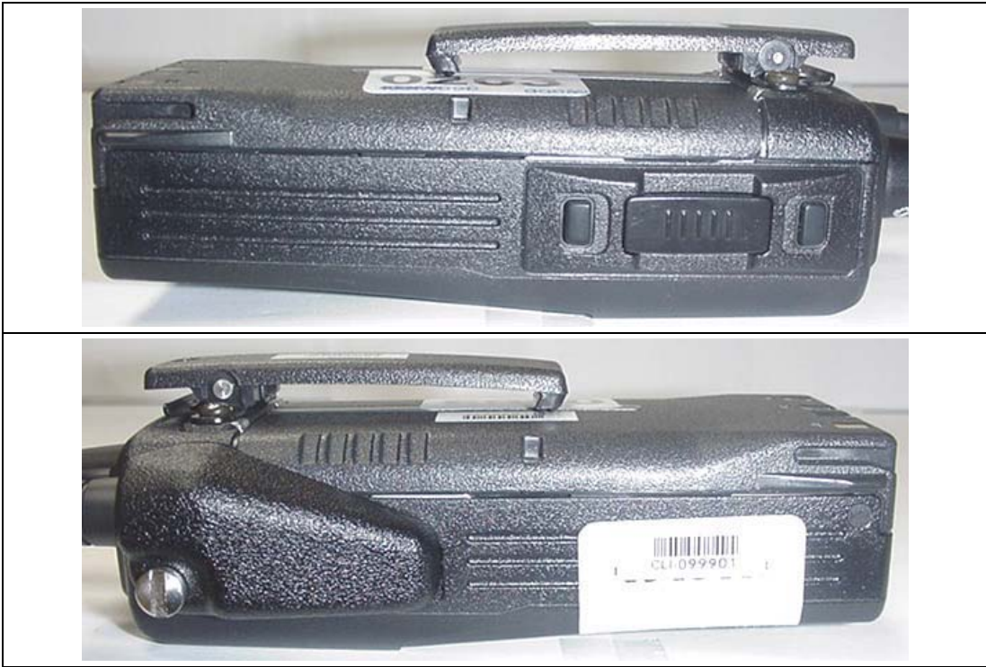
Left & Right Sides of DUT with Ni-MH 1600mAh Battery P/N: KNB-21N & Belt-Clip accessory P/N: KBH-10
