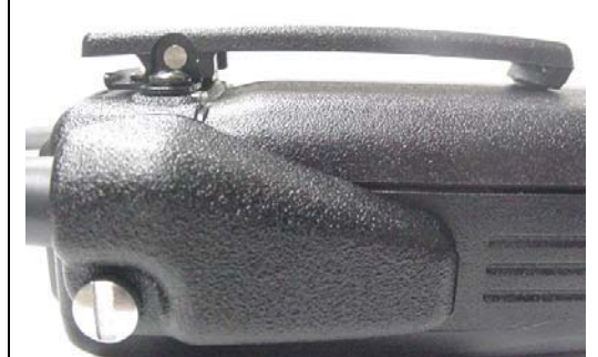
Left & Right Sides of DUT with Alkaline Battery Case P/N: KBP-4 and Belt-Clip accessory P/N: KBH-10
