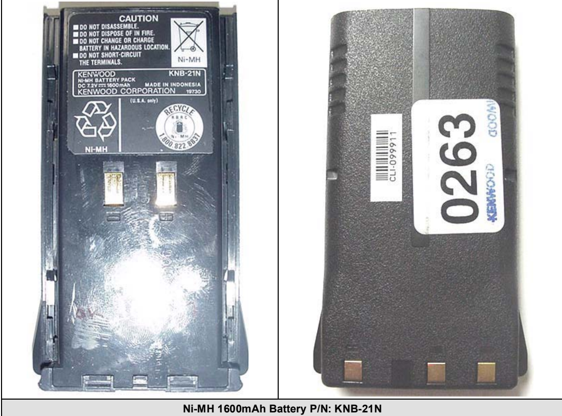
Left & Right Sides of DUT with Ni-MH 1600mAh Battery P/N: KNB-21N & Belt-Clip accessory P/N: KBH-10
