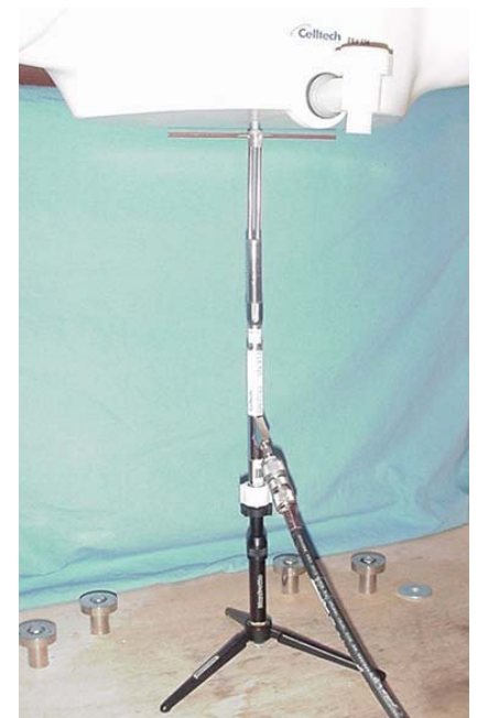
835 MHz Validation Dipole Setup
